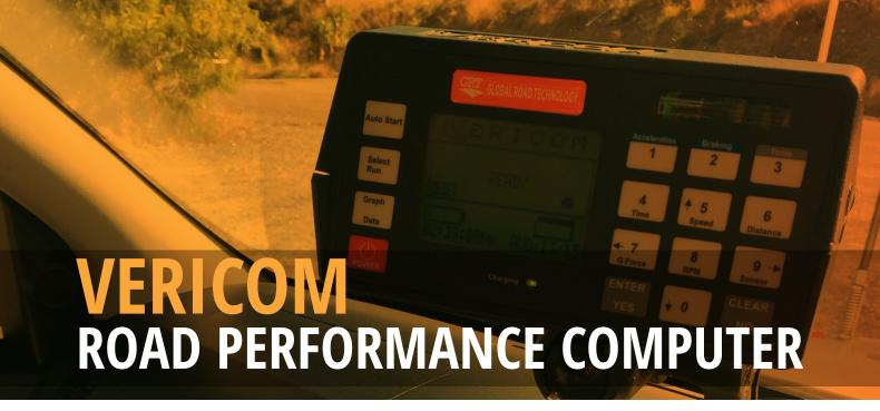
Global Road Technology (GRT) is the exclusive Australian distributor for Vericom Computers. The Vericom Computer is an electronic accelerometer / decelerometer that is capable of measuring G force, friction and designed for vehicle brake testing, acceleration and performance testing for a variety of applications for Road Agencies, organisations and companies involved in road safety, management and reporting activities.
